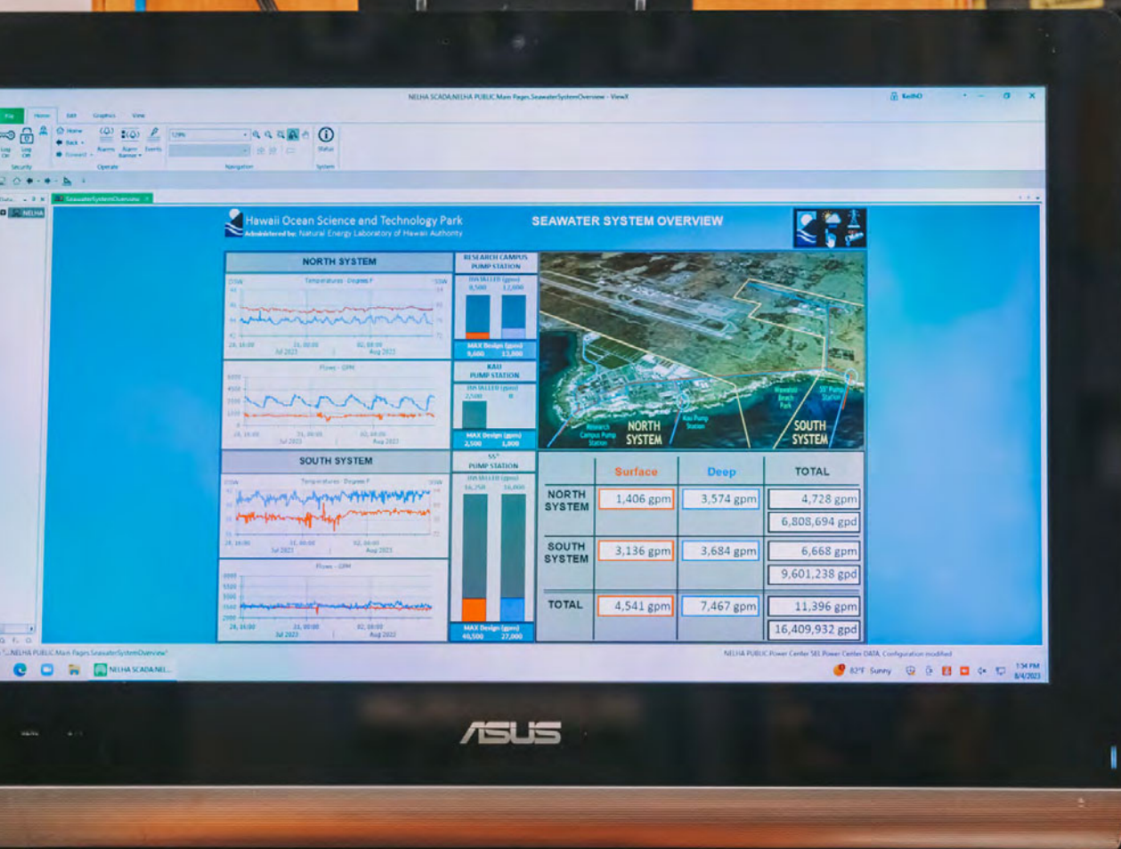
TRACKING THE FLOW: NELHA's SCADA (or Supervisory Control and Data Acquisition) system monitors how much seawater is pumped throughout the 870-acre tech park. There are three pump control stations with this one at the Keena Hana Administration offices. Photo Credit: Tetrachrome
