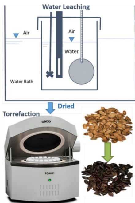
Figure 22. Laboratory scale leaching and torrefaction test equipment.
