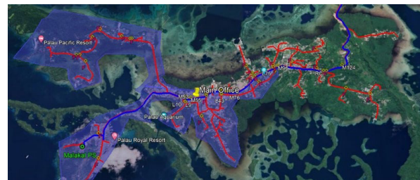
Figure 3. Distribution feeders on Malakal Island, Palau.
