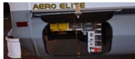
Figure 9. Bus export power unit.
