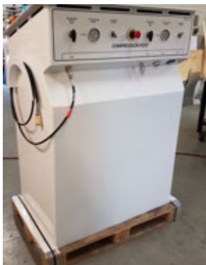
Figure 7. MTA boost compressor fueling post.
