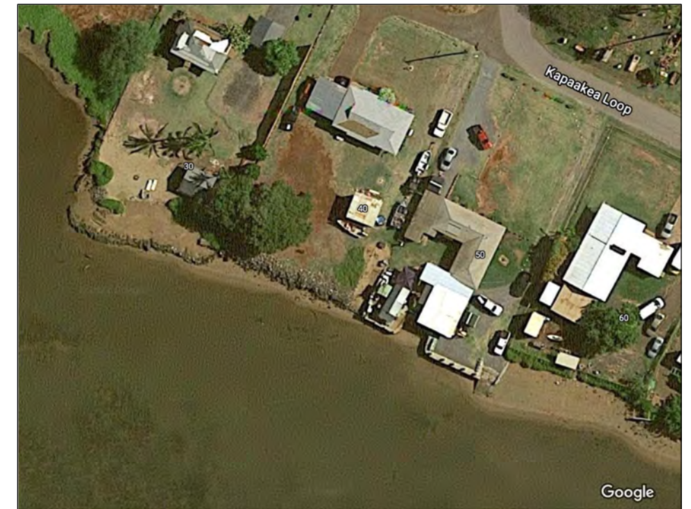
Photo: A low rocky mound at the western end of Kapa'akea forms a sill that breaks waves and captures sediment which helps to build a sandy shoreline.
