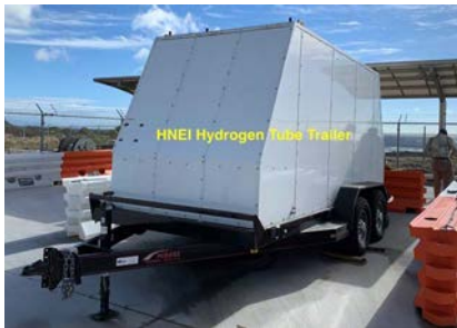
Figure 5. Hydrogen transport trailer.
