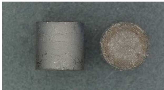
Figure 1. Biocarbon pellets produced from TPP biochar.
