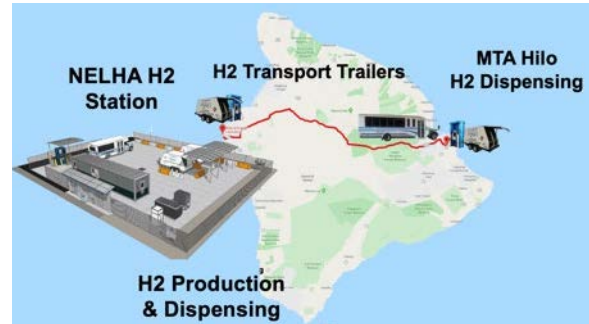
Figure 2. Concept for hydrogen transport on Hawai'i Island.
