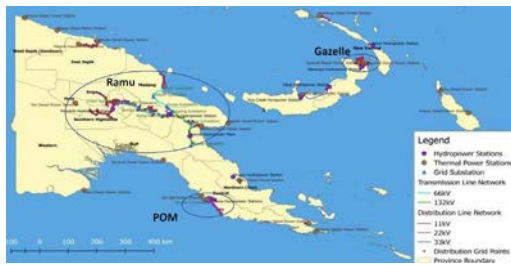
Figure 1. PPL’s Main Power Systems, extracted from the PPL Diagnostic Assessment Report submitted in 2022.
