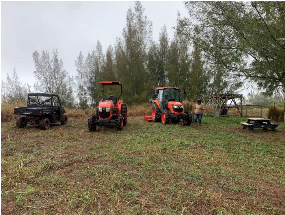
Figure 2. Starting from left to right, the Polaris Ranger, Kubota with rotary mower, Kubota with flail mower.
