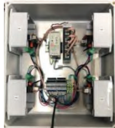
Figure 2. Load measurement box with ARGEMS devices.
