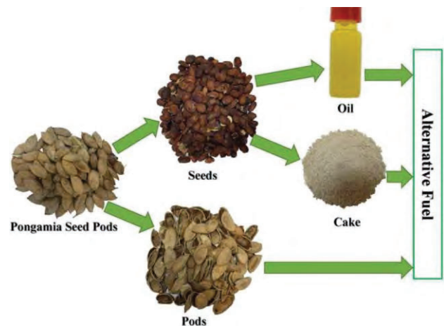
Figure 8. Pathways from Pongamia seed pods to fuel.
