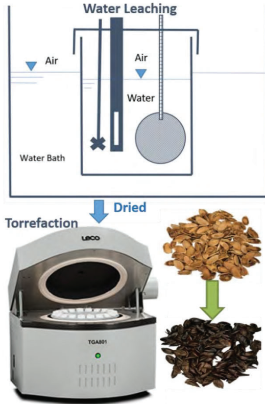
Figure 9. Laboratory scale leaching and torrefaction test equipment.
