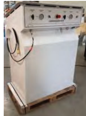
Figure 7. MTA Boost Compressor Fueling Post.
