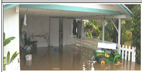
For decades residents of Wailupe Place have been plagued with flooding. Heavy rain combined with a high tide, caused an old storm drain pipe to back up. In extreme cases flooding was over 3 feet.
