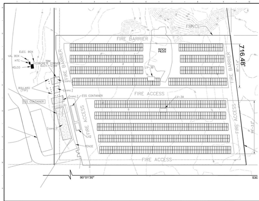
Proposed layout of the 500kw PV farm and ESS storage at the 55" pump station.
