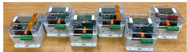
Figure 2. ARGEMS patented custom power meter and controller devices.
