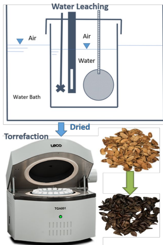
Figure 9. Laboratory scale leaching and torrefaction test equipment.
