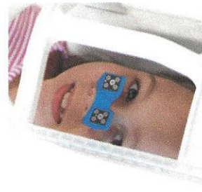
KinetiCor MRI technology for patient motion control, invented at UH Medical School 2013.
