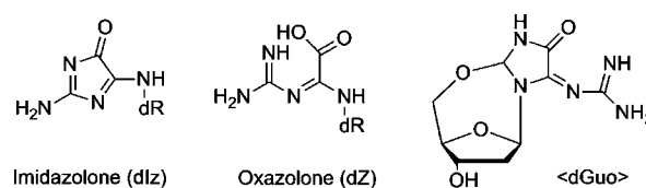
FIGURE 14. Structures of imidazolone and oxazolone, the typical product for BP-photosensitized type I oxidation of dGuo, together with the intrabase product <dGuo>.
