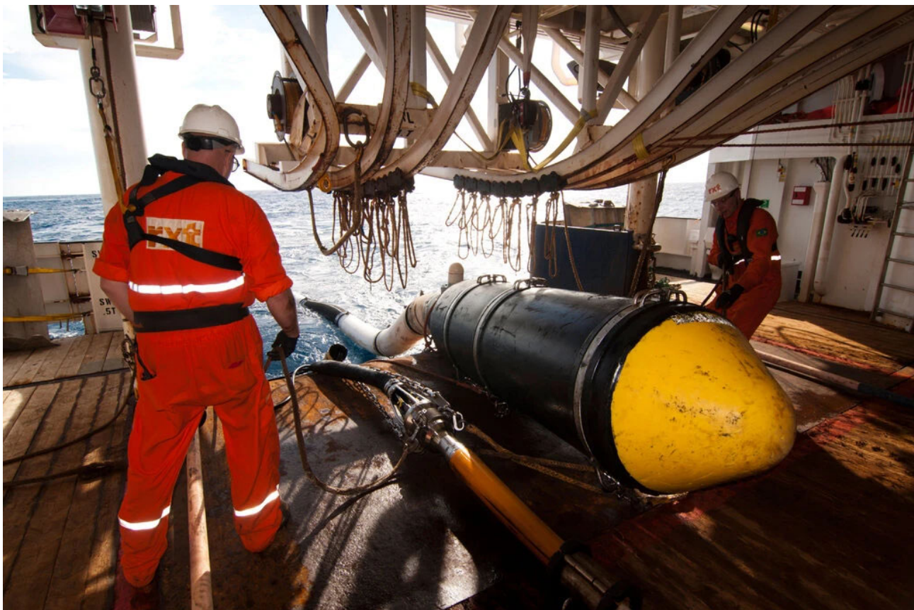
Seismic air guns on a seismic vessel in waters off Brazil. Leo Francini/Alamy
