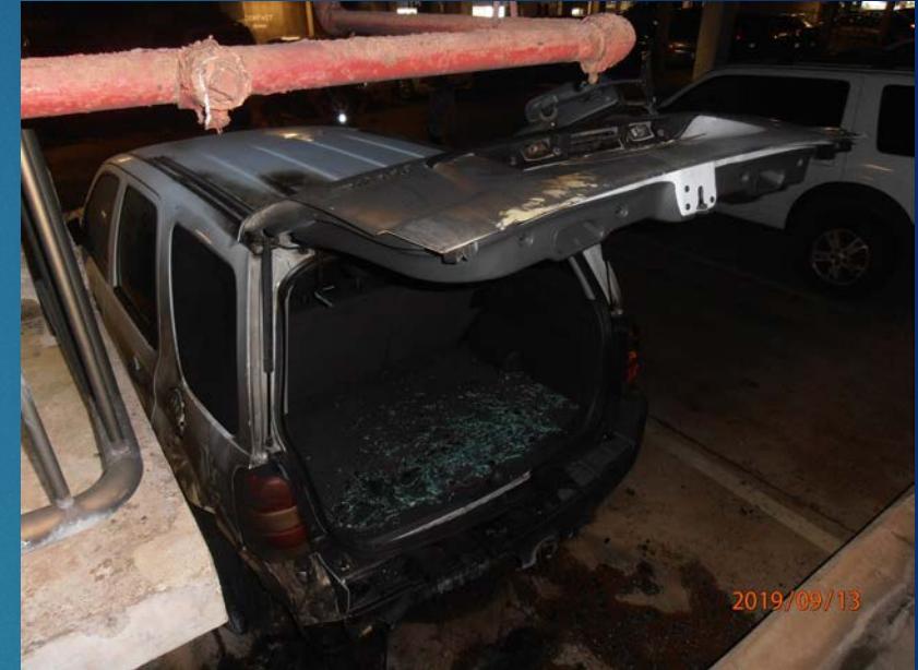
Burnt State vehicle under failed sprinkler head
