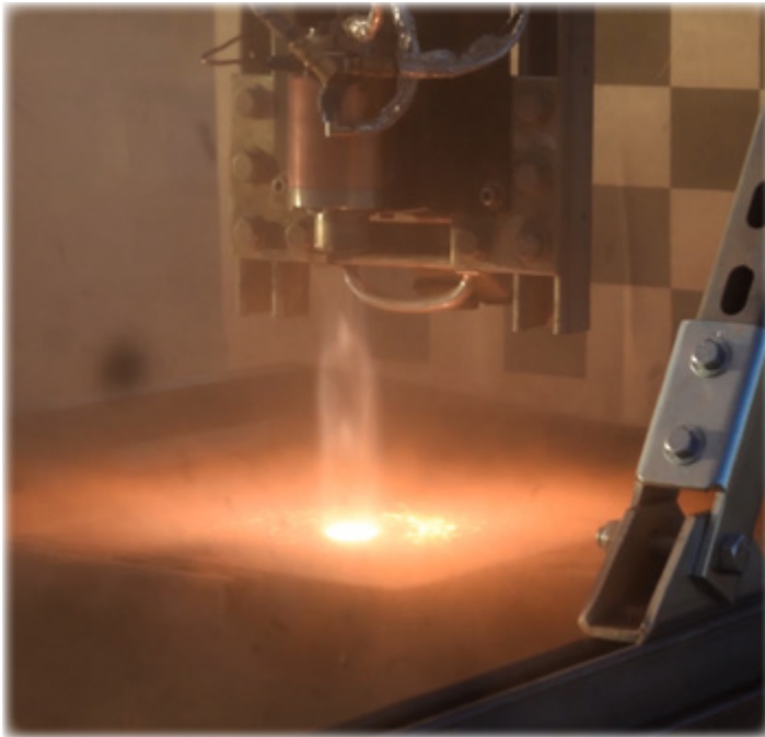
Above left: Masten Space Systems conducts a static rocket fire test of a sintered basalt landing pad tile made at PISCES. Source: Masten Space Systems. Right: Sintered basalt tiles created using only Hawaiian basalt aggregate and heat.
