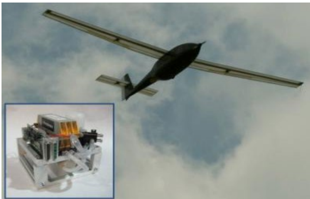
Figure 1. NRL IonTiger in flight and 550W fuel cell (insert)
