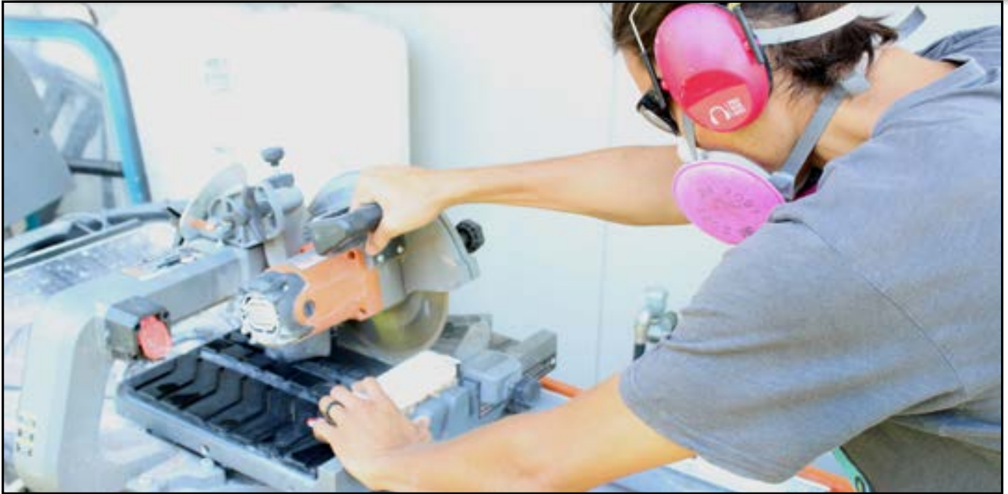
PISCES Intern Kye Harford uses a wetsaw to cut a block of sintered basalt into tiles.
