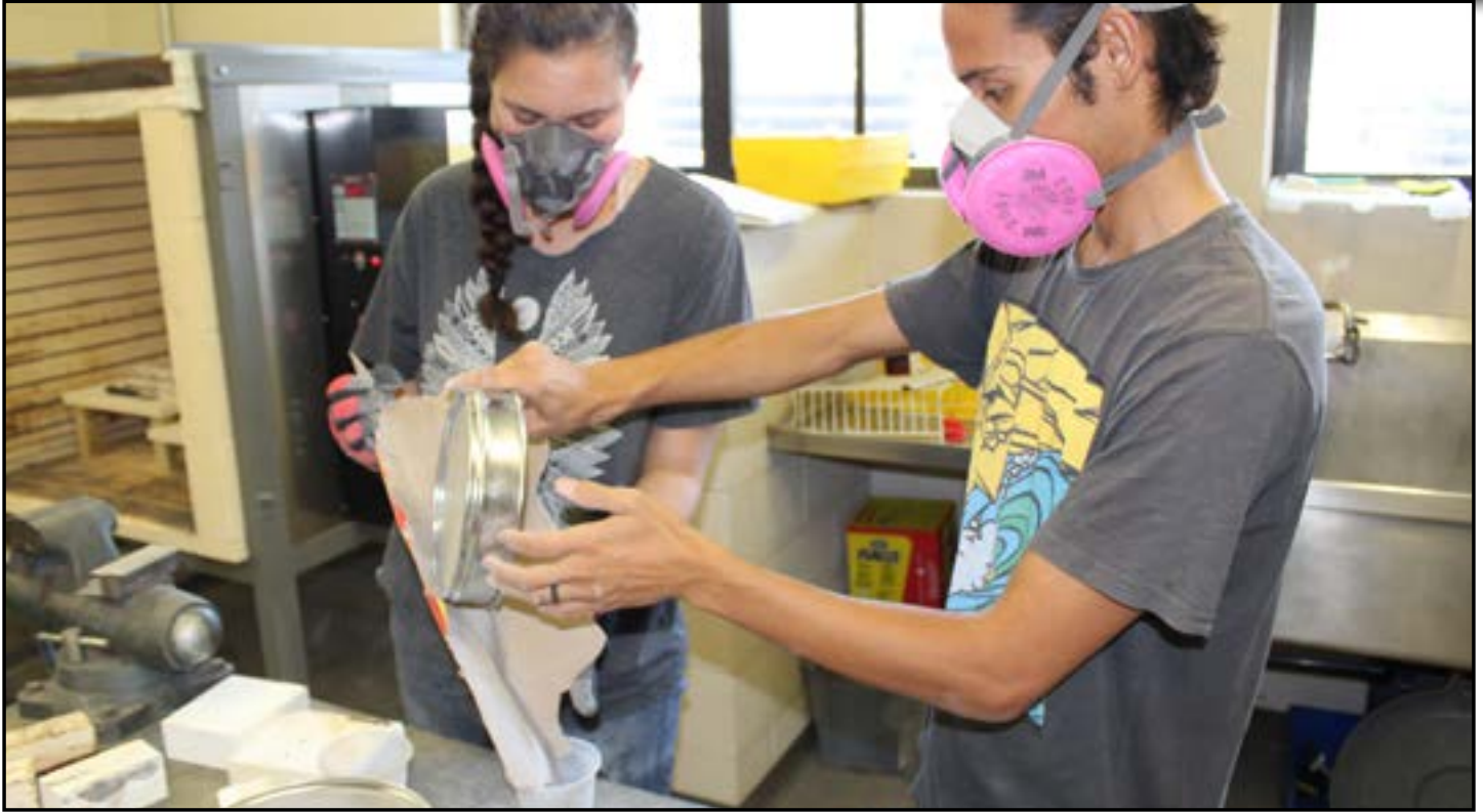
Above: PISCES Geology and Materials Science Technician Kyla Edison and Intern Kye Harford sift raw basalt fines from a local quarry before pouring them into a mold for sintering.
