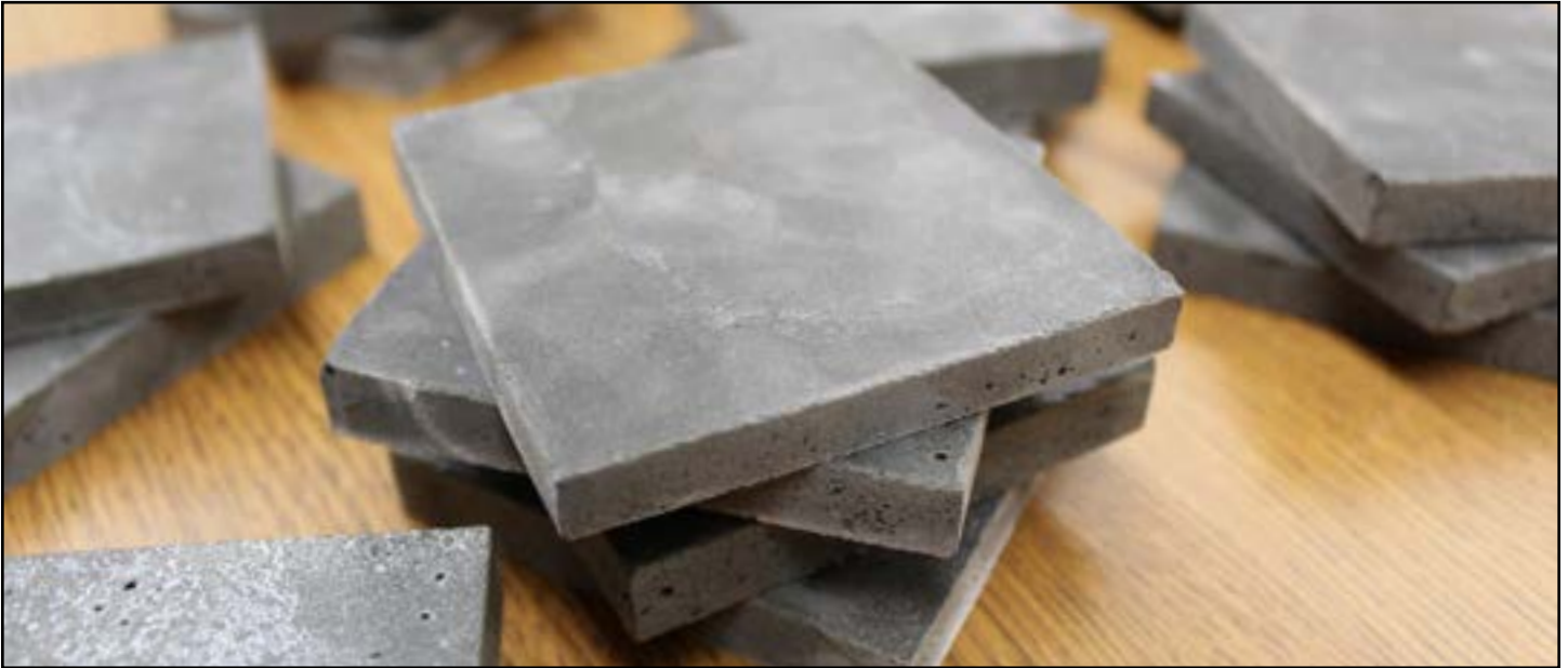
Sintered basalt tiles are made using raw basalt fines with no additional additives.
