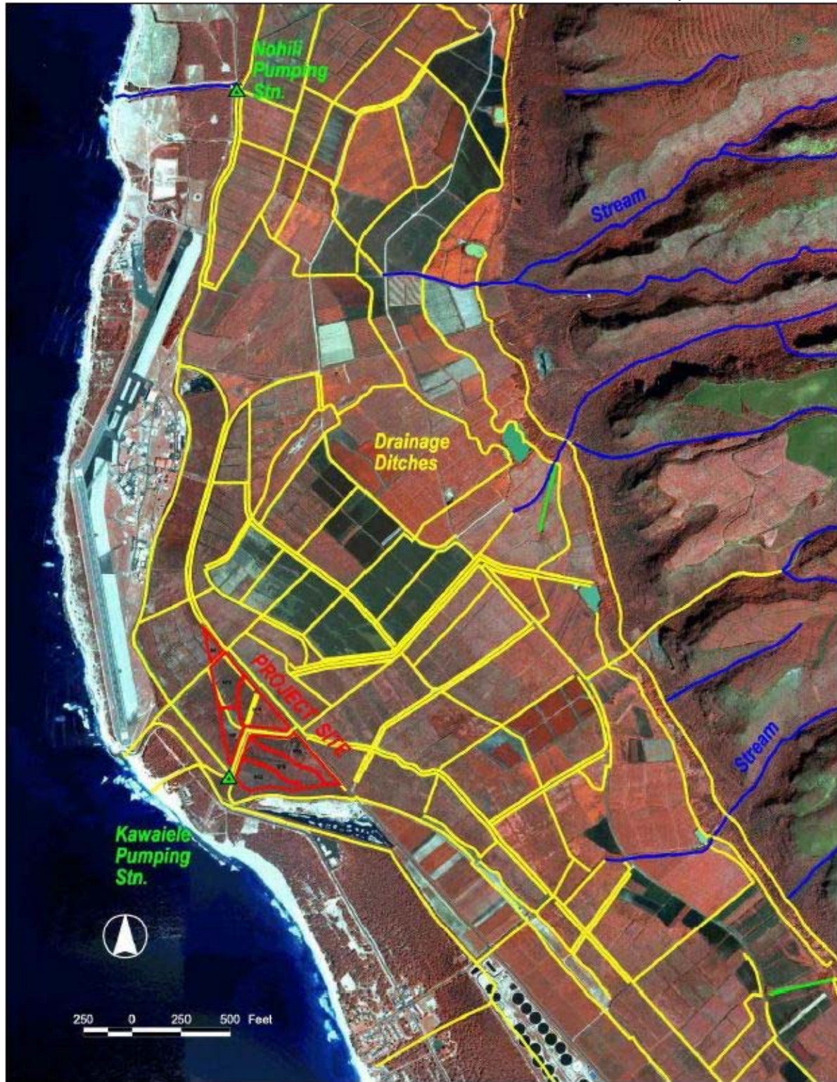
Fig. 5. Mānā Plain Drainage Ditch System and Pump Stations (Source: Final Environmental Assessment Mānā Plain Wetland Restoration Project)
