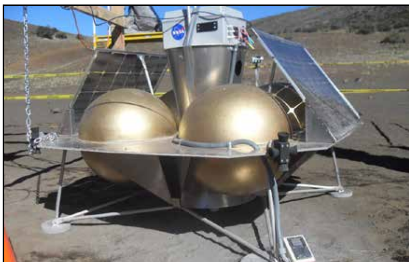
Right: A scaled-down model of GLXP team Astrobot's spacecraft during a field test on Hawaii Island in March 2015. The mock-up was built by 'Iolani High School students to test NASA's EDS technology.
