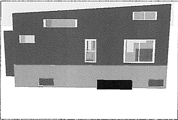
Back Side (11-windows; 9 sliders, 1 fixed, 1 single-hung)
