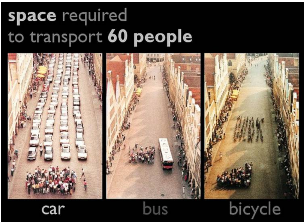
Fig. 1.0. Example of road space savings and increased road capacity through a multimodal approach.
