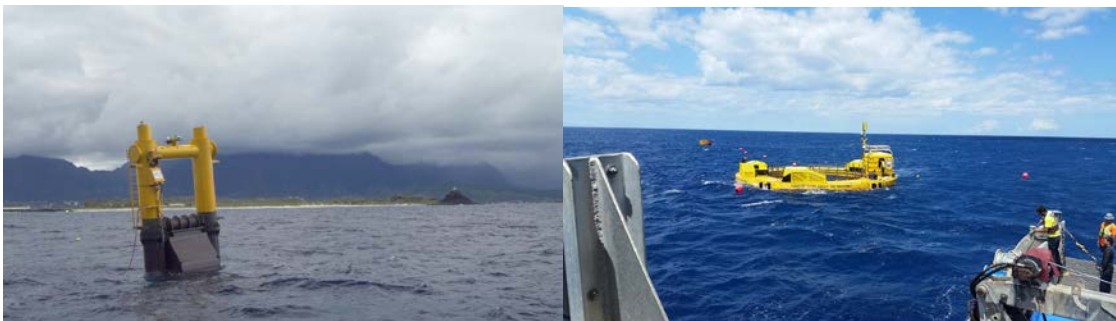
Figure 5. Azura and Lifesaver wave energy converters deployed off of Marine Corps Base Hawai'i.
