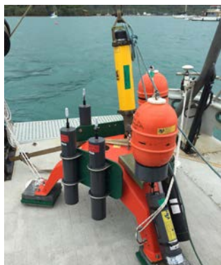
Figure 6. Acoustic device deployed at wave energy test site.
