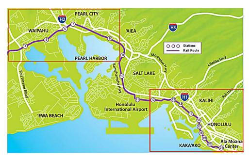
Boxed in RED show the HART rail route sections most affected by floods, tsunami, hurricane storm surge and sea level rise.
