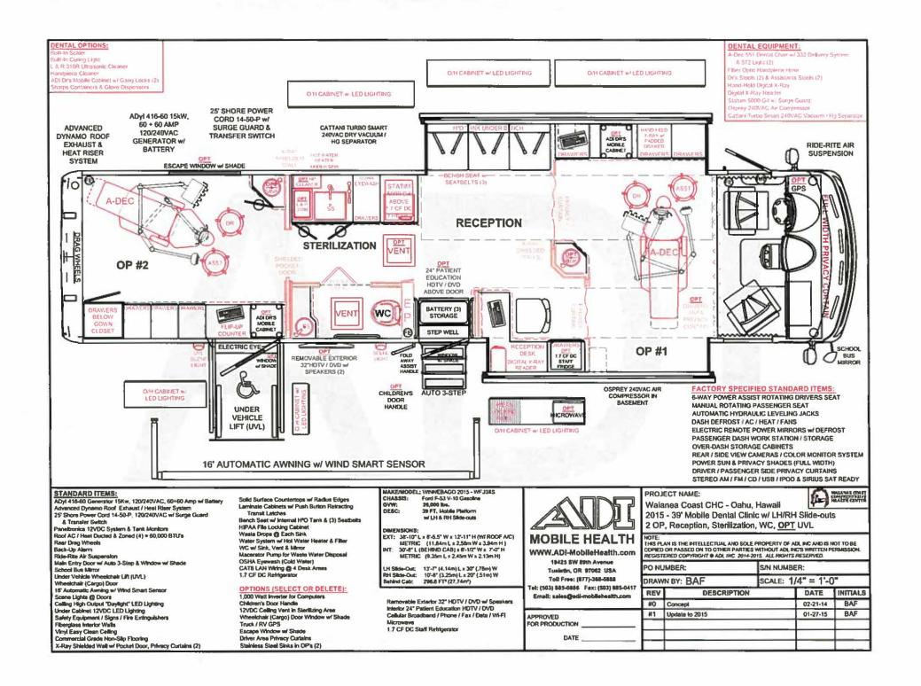
Attachment B: Dental Expansion Floor Plan
