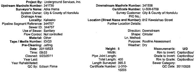
Additional Information: IDIQ3 Area A Kakaako. Note: PACP doesn't have a code for TCP. Hole in pipe. Fractures. Deposits. Patch repair. Grease in lateral.
