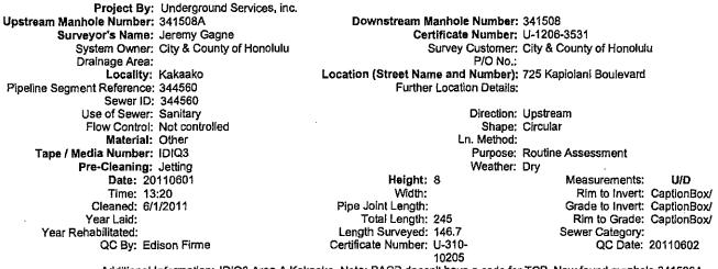
Additional Information: IDIQ3 Area A Kakaako. Note: PACP doesn't have a code for TCP. New found manhole 341508A. Camera underwater. Multiple holes in pipe. Deposits.
