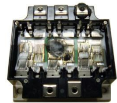
Semiconductor switch failure
