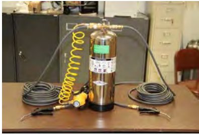
A modified fire extinguisher dubbed the "Ant-stinguisher" useful for larger scale control applications
