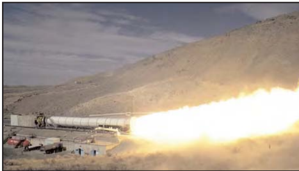
Five-Segment Motor Test
