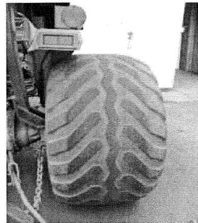
Mower tires are in need of replacement. Left tire has patches of rubber missing and right tire has worn tire tread.
