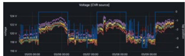
Figure 2. Voltage profiles with CVR on and off. The tap position (blue) at 0 indicates CVR is off.
